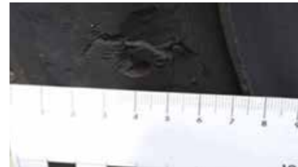
Banden: Nok > 3 mm diep, demontage
